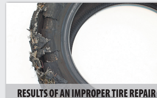
RESULTS OF AN IMPROPER TIRE REPAIR
